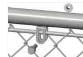
Rail & mesh connecting
